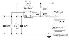
Note: Pin 1 = No connection on non tri-state models
